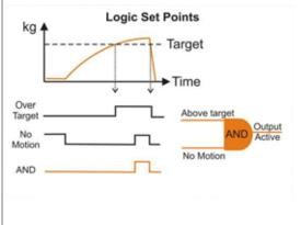
R400 Logic set points are based on the status of the inputs and the defined mask that is used to match IO1-IO24 for the logic set points.
